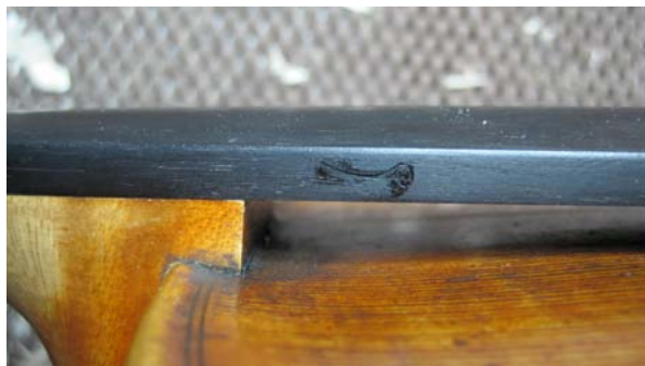
(The finished project. The cardboard insert is now between the neck block and the top plate. The repair is almost invisible.--ed)
